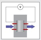
The MSRS responds quickly to oxygen and has a T90 of under 11 seconds. Another benefit of having a sealed reference is that measurements can be made without a reference gas and independent of the quality of the surrounding air. The analyzer is virtually drift-free, extending calibration interval time.
