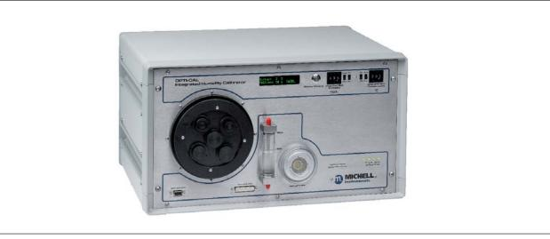
The OptiCal is a premium calibration solution for humidity sensors. The stand-alone and transportable calibrator requires no external services other than mains power, and features an integrated chilled mirror reference instrument to enable the operator to perform calibrations that are traceable to national standards.
