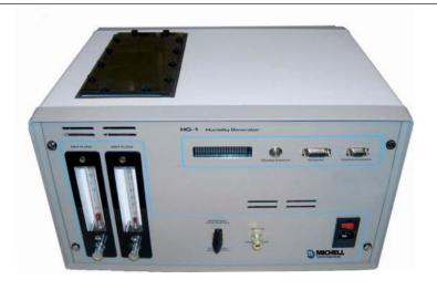
A low-cost, easy to use, fully integrated system for the calibration of dew-point and relative humidity sensors from 2 to 90% relative humidity, -30 to +20°Cdp (-22 to +68°Fdp).
